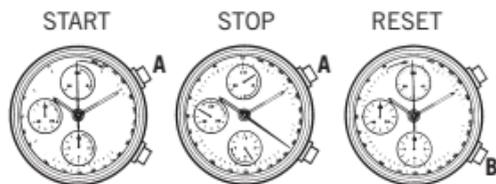
3. To use the chronograph, push the button at 2 o'clock once. The second counter will start counting. To stop the chronograph at any time, push the button at 2 o'clock once again.
