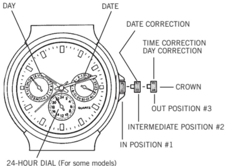
1. Pull the crown out to position #3. Move the hands forward by turning the crown. The date changes at midnight and the day of the week will change after the date. Keep moving the hands forward UNTIL THE CORRECT DAY OF THE WEEK SHOWS ON THE DAY HAND. Then set the hands to the correct A.M. or P.M. time. Push the crown back in to position #1.
