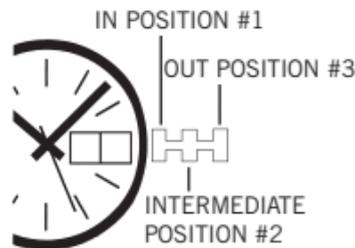
1. Pull out the setting crown to position #3. Move the hands forward by turning the crown. Observe the date as the hands move past 12 o'clock. When the date changes it is midnight on the watch. Set the hands to correct A.M. or P.M. time. Push the crown back in to position #1
