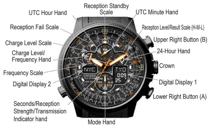
NOTE: Under normal conditions, this watch will receive radio signals to automatically update the time and calendar. There may be conditions in which the radio signal cannot be received. If a signal cannot be received, the watch will operate normally, but not update.
