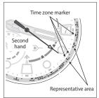
On the illustration in the left, the second hand points to 21 seconds and time zone setting is "+9"
